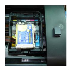
Ciss with original cartridge. The ciss uses the Original cartridge signal to fool the printer into thinking all the cartridges are original.
