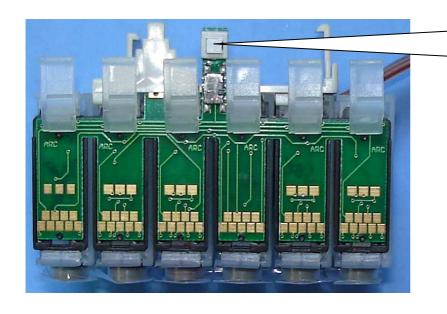
Reset Switch to make printer recognise the cartridges
